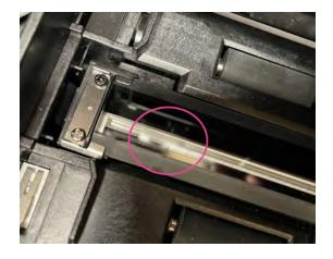
There was one fairly significant ink smudge, shown twice in the photos above. Its position corresponds to the location of the most pronounced streak on the ballot images. There were also a couple smaller smudge marks which presumably align with the lesser streaks shown in the images. The streaks were easily removed with a microfiber cloth used for cleaning eyeglasses. Given this, we're confident that the issue is fixed by cleaning the sensor glass.
